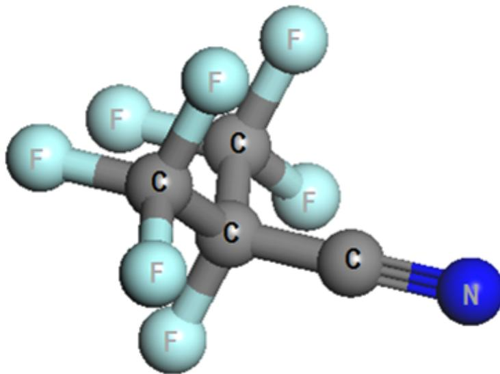
*Novec<sup>TM</sup> 4710: A new compound developed specifically by 3M<sup>TM</sup> for dielectric applications, fluorinated nitrile*
